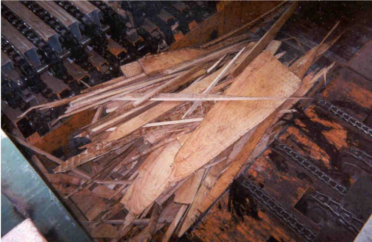
Figure 5.5 – Sawmill Downfall (Slabs and Edgings) Staged for Feeding into an OSB Disc Strander
