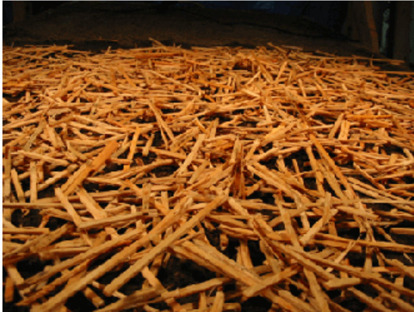
Figure 6.15 – Woodstraw™ Erosion Control Mulch
