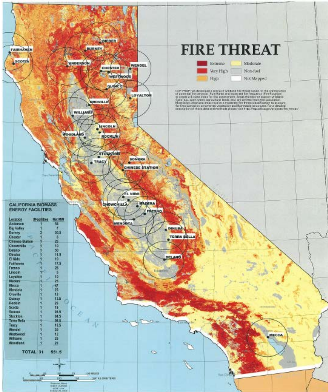
Figure – 3.8 California’s Biomass Energy Industry (circa 2008) and Fire Threat (circles around each plant represent the economically feasible haul distance)
