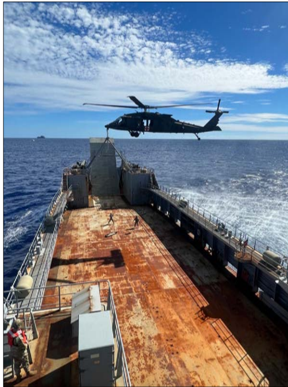
Figure 2. An HH-60M MEDEVAC Black Hawk helicopter executes hoist iterations to Army Logistics Support Vessel 3, which is traversing the open ocean south of Honolulu, Hawaii, at 5 knots (Source: Mahdi Al-Husseini / ©2024 Mahdi Al-Husseini)
